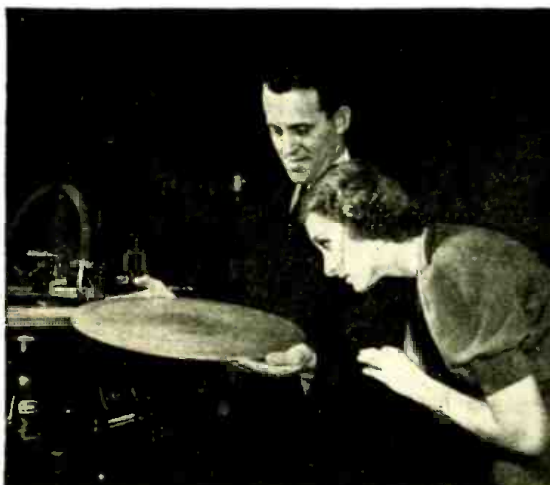
3 —WAX DISK—Next a visit to the recording room, where the stylus has done its work on the nice new wax disk. The engineer hoists the disk off the machine and Miss Blackburn takes a gander at it. The program is all waxed now.
