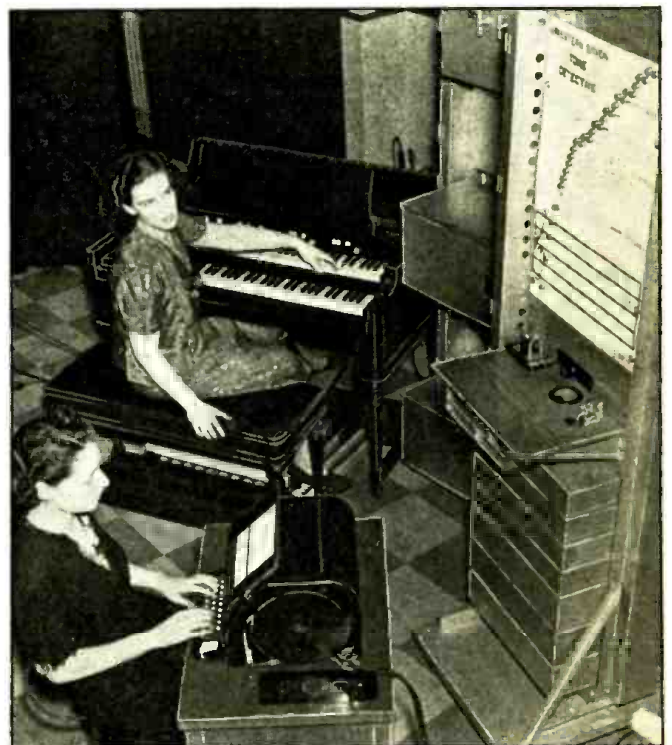
While concert organist Virginia Oman produces a single musical tone on the electronic organ, the operator at the left "codes" the tone with the telegraph message. The tone then goes over regular line along with many others. The tone produced is visually indicated by a pilot bulb on the musical scale of the "Tone Detector" shown at upper-right.
