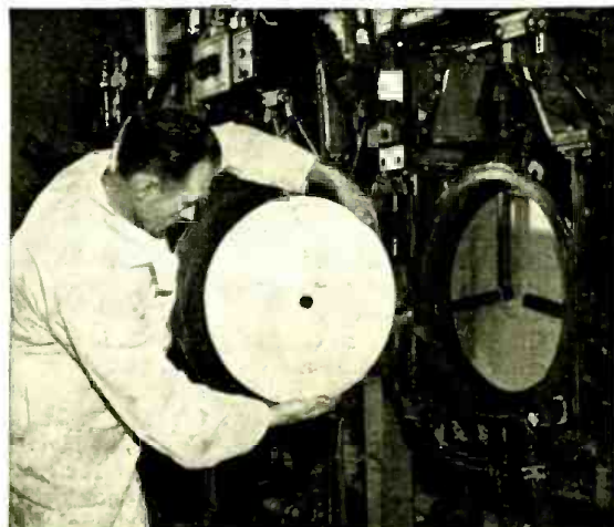
5 —COPPER DEPOSIT—After gold, comes copper. The gold-plated disk goes into a solution of copper sulphate. In due time it comes out again, with a layer of nice new copper on top of the gold. Then it goes into this machine, and a thick layer of copper is deposited on its surface.
