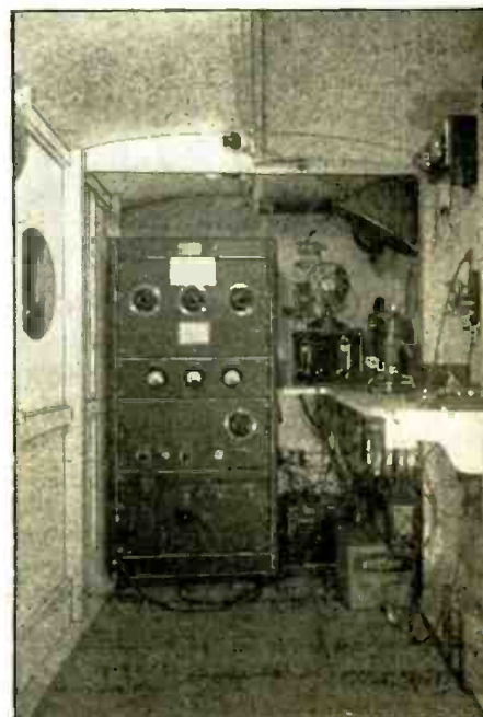
The radio, and line-telephone and -telegraph equipment are powered by optional generator or storage battery.
